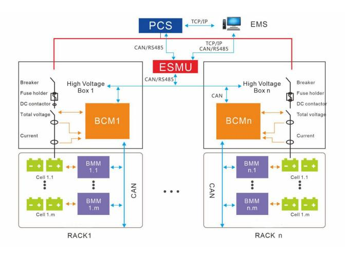
The above schematic shows GOLD ELECTRONIC's BMS architecture from the module level. The relationship of BMS, PCS and EMS, also the communication mode of them.
